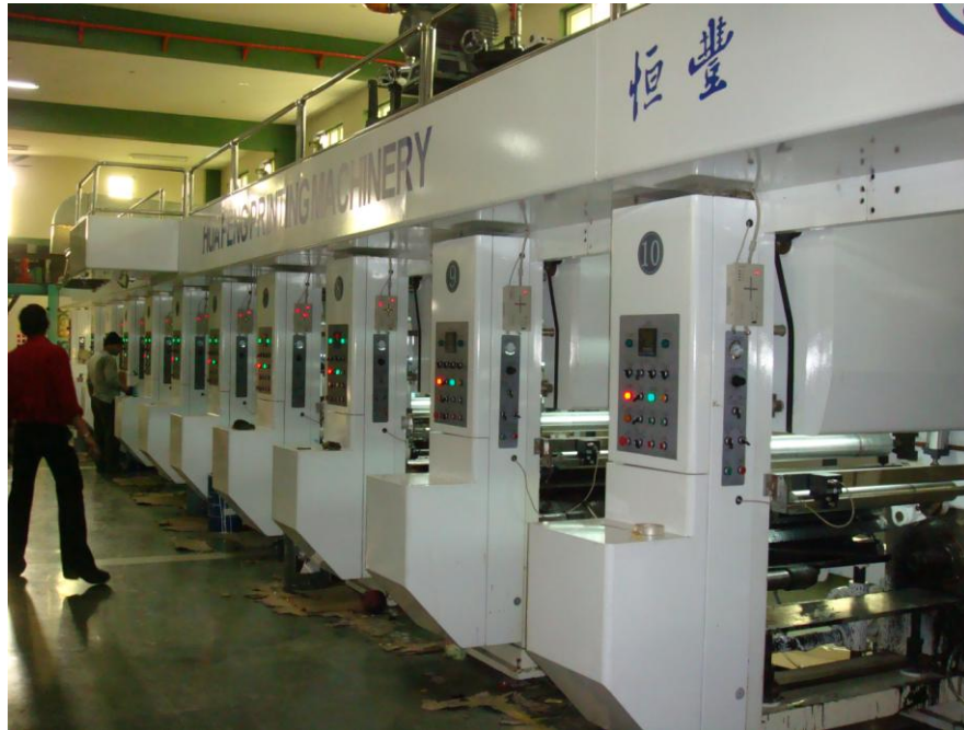
RotoGravure Printing Machinery at our Greater Noida facility
